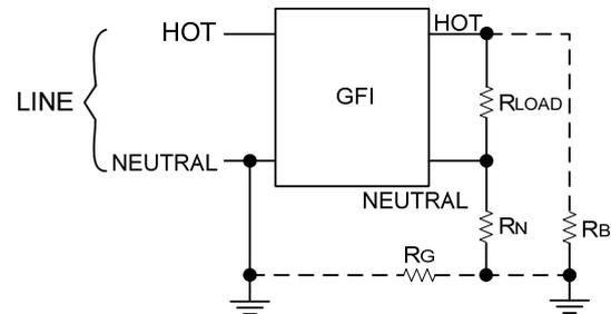
**Grounded Neutral Fault:** An unintentional electrical path between the load terminal of the neutral line and the ground, as shown by the dashed lines.
