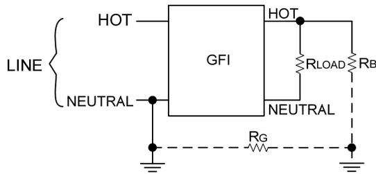
**Normal Fault plus Grounded Neutral fault:** The combination of the normal fault and the grounded neutral fault, as shown by the dashed lines.
