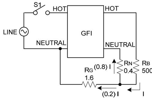
UL943 specifies  $\leq 25$  ms average trip time under these conditions. Calculation of  $C_t$  based upon charging currents due to normal fault only is as follows:
