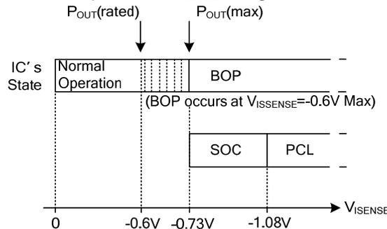
Fig. 8 BOP, SOC and PCL Protection as Function of  $V_{ISENSE}$
