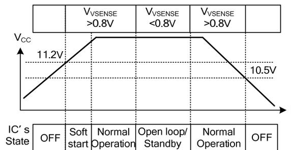
Fig. 3. State of Operation Respect to  $V_{CC}$
