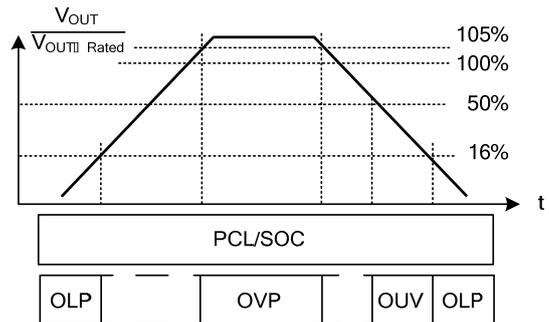
Fig. 7 V<sub>OUT</sub> Related Protection Features
