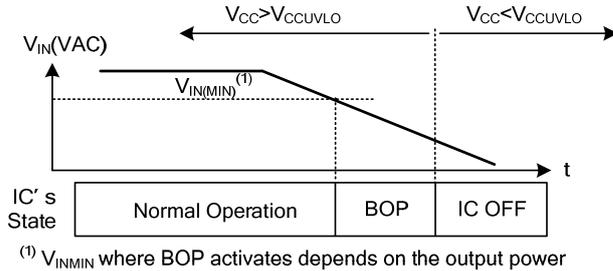
Fig. 6 V<sub>IN</sub> Related Protection Features
