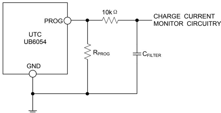
Fig1. Isolating Capacitive Load on PROG Pin
