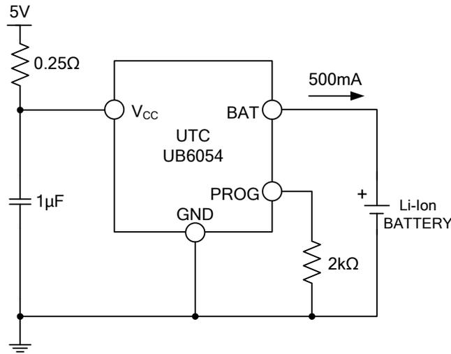
Fig3. 500mA Li-Ion Charger with External Power Dissipation
