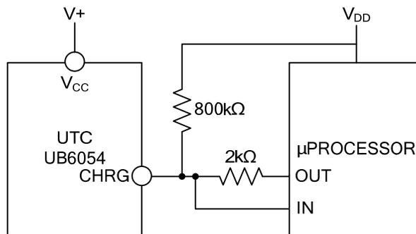
Fig3. Using a Microprocessor to Determine CHRG State
