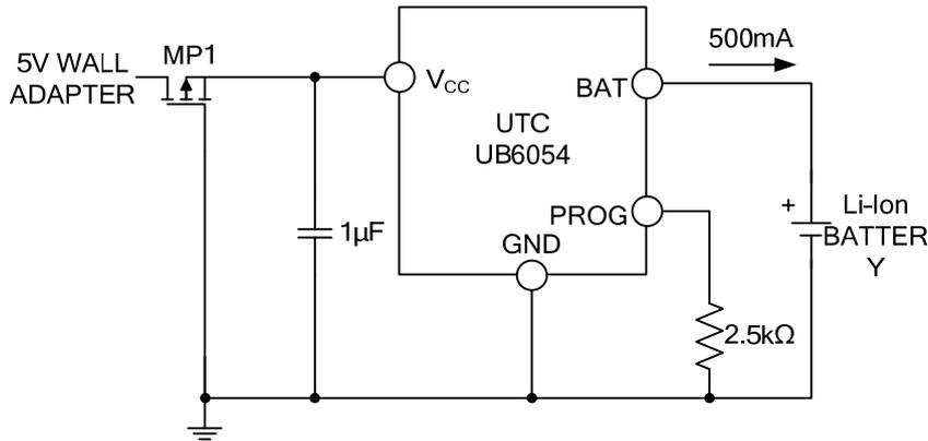
Fig4. Low Loss Input Reverse Polarity Protection
