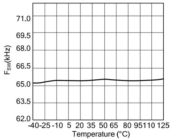
Frequency in Power-Saving mode ( $F_{SW-Power-Saving}$ ) vs Temperature
