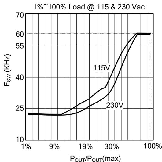
Fig.1 The relation curve between f<sub>sw</sub> and relative output power POUT/ POUT (MAX)
