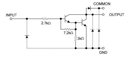
Note: The input and output parasitic diodes cannot be used as clamp diodes.
