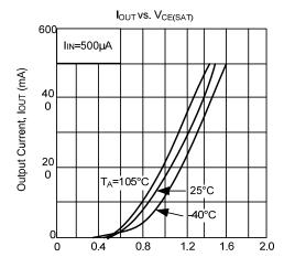
Collector-Emitter Saturation Voltage,  $V_{\text{CE(SAT)}}\left(V\right)$
